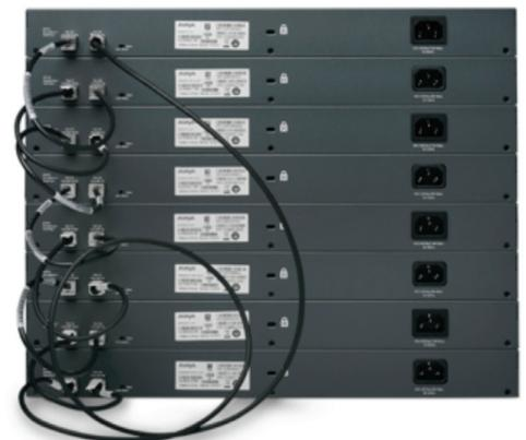
Figure 4: Avaya ERS 3500 in an eight unit stack
