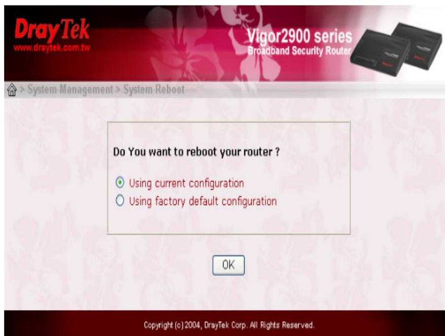
There are two reboot options: **Using current configuration** and **Using factory default configuration**. If you want to reboot the router using the current configuration, check **Using current configuration** and click **OK**. To reset the router settings to default values, check **Using factory default configuration** and click **OK**. The router will take 3 to 5 seconds to reboot the system.
