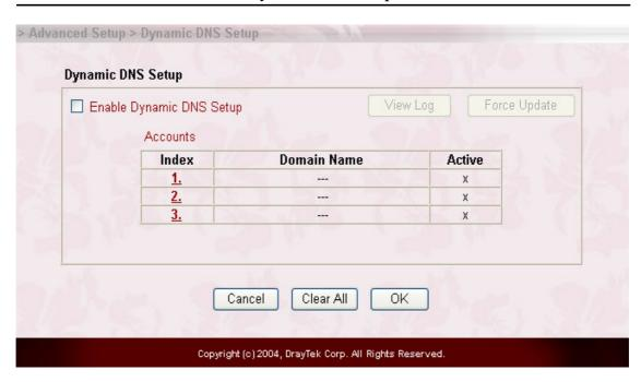
3. Check **Enable Dynamic DNS Setup** and Index number **1** to add an account for the router.
